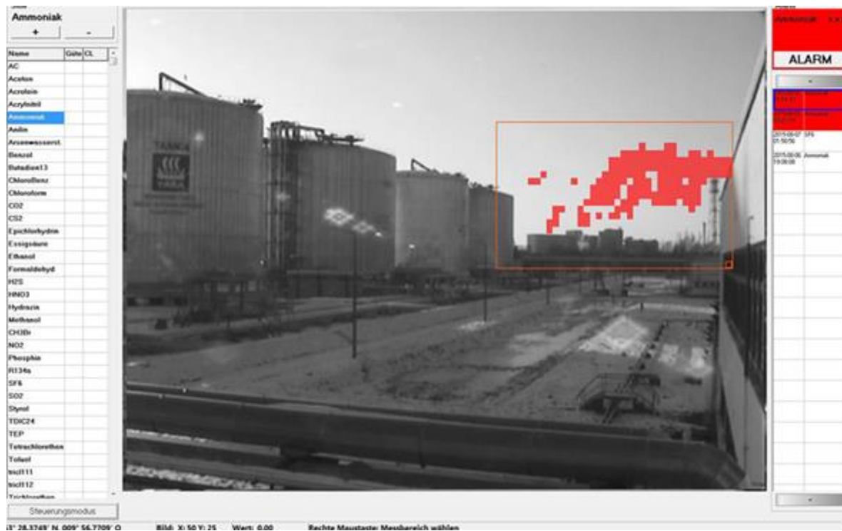
Screenshot of the OPUS RS software: The system automatically identifies and visualizes an ammonia cloud. The plant operator is warned visually and acoustically. The screenshot shows the video image of the scenery and marked orange the scan area. On the left the target library is displayed, all compounds in this list are searched for automatically within each measurement.
