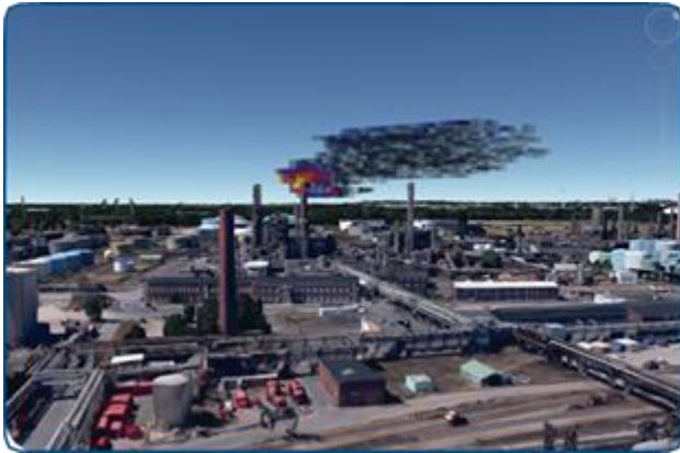
3-Dimensional distribution of an ammonia cloud around an emission stack calculated from the tomographic reconstruction of the simultaneous measurement of the cloud with two SIGIS 2 systems (viewed in Google Earth™, light colors indicate high concentrations, dark colors low concentrations)
