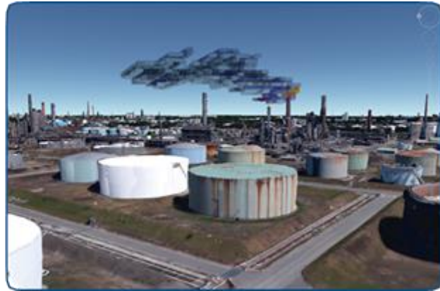
3-Dimensional distribution of an ammonia cloud around an emission stack calculated from the tomographic reconstruction of the simultaneous measurement of the cloud with two SIGIS 2 systems (viewed in Google Earth™, light colors indicate high concentrations, dark colors low concentrations)
